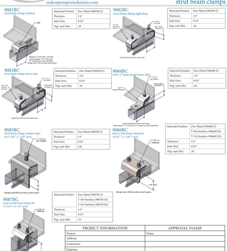
Design load 1200 Lbs when used in pairs.
